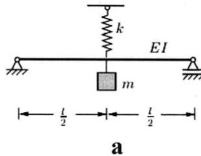
$$\omega_b = \sqrt{\frac{k + \frac{4\lambda EI}{l^3}}{m}}, \quad \omega_a = \sqrt{\frac{k \left( \frac{4\lambda EI}{l^3} \right)}{m \left( k + \frac{4\lambda EI}{l^3} \right)}} \quad (1)$$
